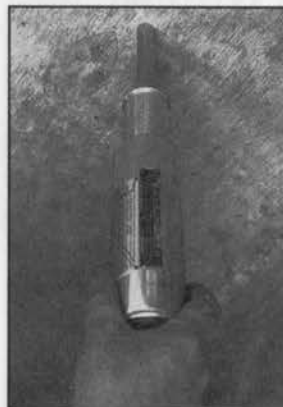
Rebound Test (ASTM C805)
